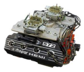
750HP @ 6500 RPM 700 TORQUE @ 5200 RPM 4.500" BORE 4.500" STROKE RAN W/ BRAD PENN 30WT BREAK-IN OIL FULLY PREPPED MOPAR/CALLIES IRON BLOCK EAGLE 4340 CRANK (4.500" x 2.200") EAGLE H-BEAM RODS (7.100" x 2.200") DIAMOND PISTONS (10.75: 1) CHROME VALVE COVERS STANDARD COMP SOLID ROLLER .704/.272/.280 MODMAN INTAKE (2x4) 2-750 CFM EDELBROCK CARBS MILODON PAN, TRAY & 1/2" PICKUP **MSD DISTRIBUTOR & ICH WIRES INDY 426 SR CNC HEADS** (2.250X 1.94 170CC) ATI BALANCER INDY ROLLER ROCKERS
